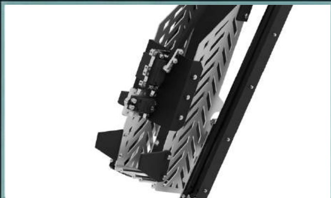
Rendered outtake. Dual-motor drive integration and optimized plate topology.
