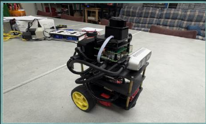
Full robot assembly. Sensor layout, cabling, and compute integration.
