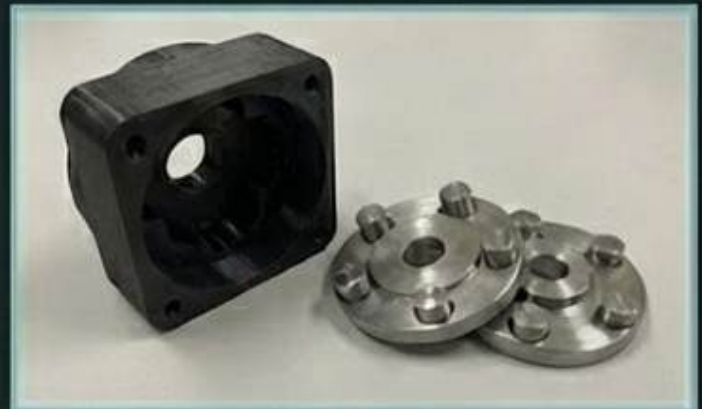
Manufacturing validation. Fit check of cycloidal lobes and housing.
