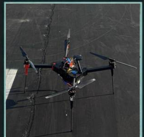
Final integrated platform – reinforced frame and field-ready configuration.
